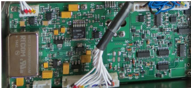
Figure 5 Fabricated & Assembled PCB for Control circuit
